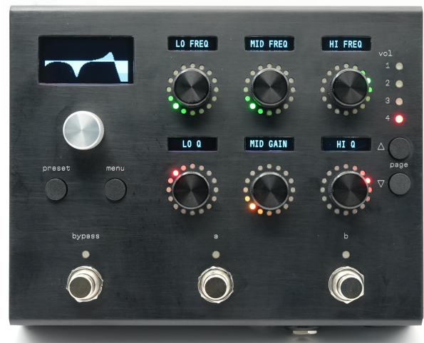
Figure 5: Top view of the graetli user interface. The depicted state shows the controls of a parametric three-band equalizer.
